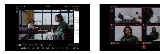
Monitor & Control (M&C) is an application that connects to a single camera and is used for remote control of the camera and to display/control clips from the camera. You can also connect to up to four cameras using the multi-camera monitoring function (iPad only). This app can be used free of charge.
