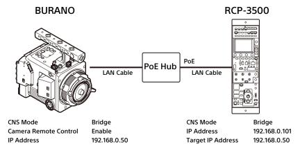
This is an example of the procedure to connect BURANO and RCP-3500.
